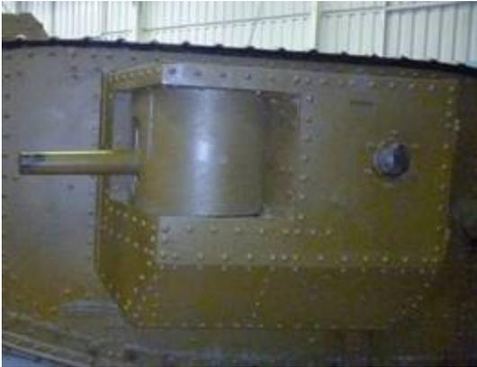
The sponsons, as can be seen in this and the previous photograph, clearly protrude, and the dimension from the outer face of the main body of the tank to the outboard face of the sponson is about 28 inches (or 71 cm). The fore and aft faces are sloped, as is the lower part of the outboard face. There are no obvious gripping points so manhandling would be difficult, if not impossible given that it was made of half-inch thick armour plate and weighed in, so I was informed, at about a ton.
